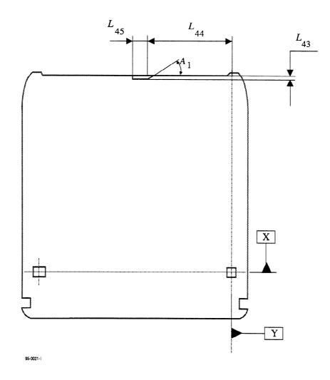
Figure 10 - Shutter sensor notch viewed from Side A
