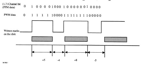
$DSV_m$  is calculated as  $DSV_m = (+5 - 4 + 8 - 5 \dots)$  2. The Resync area shall be divided into two parts (RS || INV), where both parts are concatenated as follows:
