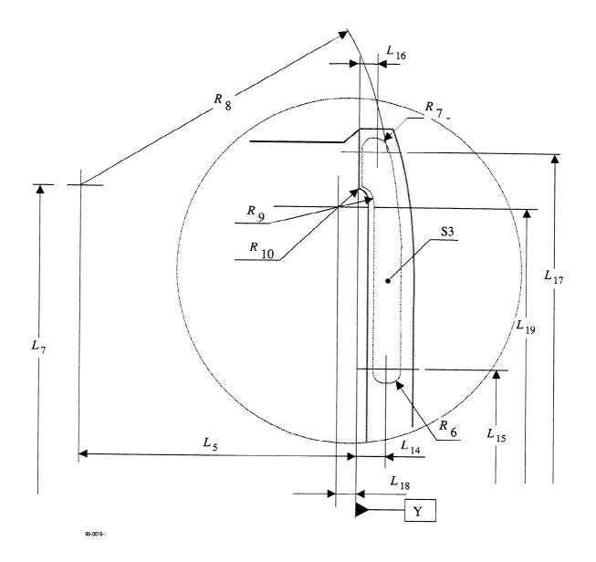
Figure 5a - Detail of surface S3
