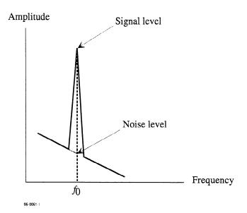
Figure 27 - Amplitude versus frequency for the magneto-optical signal
