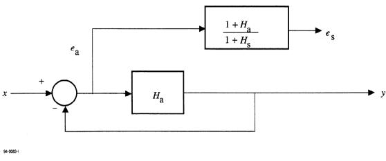
Figure T.4 - Implementation of a reference servo by changing the tracking error of the actual servo
