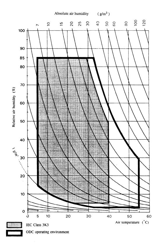
Figure Q.1 - Climatogram of IEC Class 3K3 and the ODC operating environment
